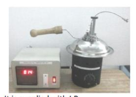
Electric heater with Energy regulator temperature control. Suitable for operation on 220 Volts A.C. 50 Hz. It is supplied with I.P. Thermometer.
