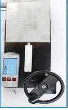
Measurement Range: The Z axis (vertical)  $\pm 80 \mu m/\pm 160 \mu m$
