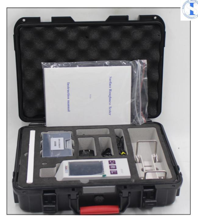
Portable Surface Roughness TesterJD520 is a high accuracy instrument for measuring surface roughness. It can be used on variety of machining parts and operates on various surfaces, not only flat but also outer cone, outer cylinder, curved, pinholes, grooves, recesses grooves and axle etc.
