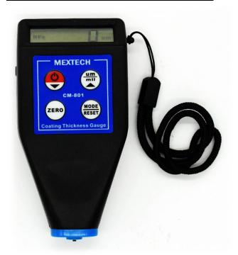
**APPLICATION:** The Fe function measure the thickness of non-magnetic materials (e.g. paint, plastic, porcelain e namel, copper, zinc, aluminum, chrome etc.) on magnetic Materials (e.g. Iron, nickel etc.). Often used to measure t he thickness of galvanizing layer, lacquer layer, porcelain enamel layer, phosphide layer, copper tile, aluminum tile, s ome alloy tile, paper etc.
