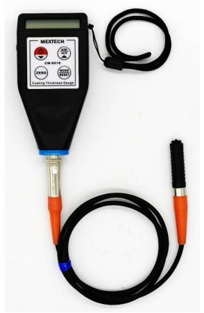
**APPLICATION:** The Fe function measure the thickness of non-magnetic materials (e.g. paint, plastic, por celain enamel, copper, zinc, aluminum, chrome etc.) on magnetic Materials (e.g. Iron, nickel etc.). Often used to measure the thickness of galvanizing layer, lacquer layer, porcelain enamel layer, phosphide la yer, copper tile, aluminum tile, some alloy tile, paper etc.
