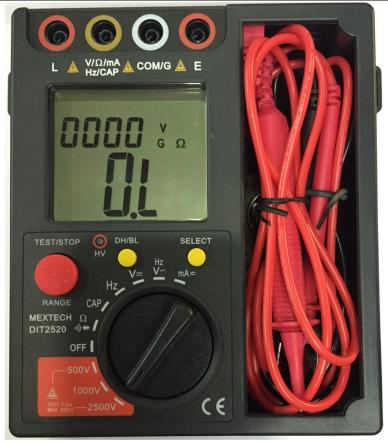
The meter with auto range selection is digital Insulating resistance tester & Digital multimeter. It has features of complete functions, high accuracy, reliability in operation.
