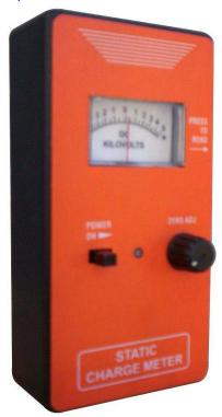
The unit gives direct readings of electrostatic potentials on any surface, when held at a distance of 2.5 cms. However, virtually any electrostatic potential can be measured by proportionately increasing the distance from the meter to the charged object.
