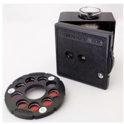
The Comparator is meant for visual determination of the colour of lubricating oils, heating oils, diesel fuel oils and petroleum waxes.
