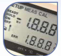
Custom dual line LCD provides optimum view of both pH and Temperature values
